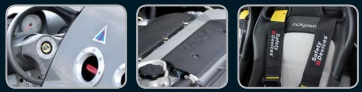
Lotus Exige Cup car: Powered by a mid-mounted 1.8 Toyota VVTL-i 2ZZ GE engine, utilising independent suspension with Ohlins 2 way adjustable dampers, adjustable anti-roll bar and limited slip differential. The Lotus Exige Cup car also has a full FIA roll cage with sports seats and four-point harnesses amongst other modifications.
