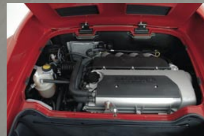
Mid-mounted, Toyota sourced, VVTL-i engine provides high-rev boost for lightweight Elise.
