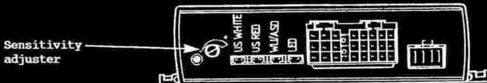
**Adjustment Procedure:** Turn off the siren (using the siren key), and use the hazard lamps as an indication of alarm triggering.
